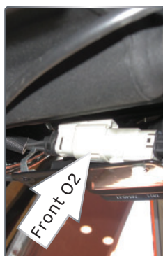
2012-2023 Softail Models The stock O2 connectors for the front cylinder are found at the front of the engine near the voltage regulator. The stock O2 connectors for the rear cylinder are found under the seat near the battery.
