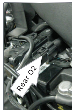
Sportster Models The stock O2 connectors for the front cylinder are always at the front of the engine on the left side near the oil filter. The stock O2 connectors for the rear cylinder are above the battery on 2014-2015 models or just rear of the engine on 2007-2013 models (not shown).
