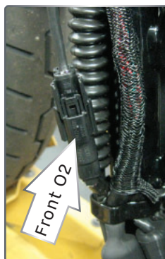
Sportster Models The stock O2 connectors for the front cylinder are always at the front of the engine on the left side near the oil filter. The stock O2 connectors for the rear cylinder are above the battery on 2014-2015 models or just rear of the engine on 2007-2013 models (not shown).
