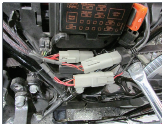
Connect the Power Vision cable to the other side of the Y-adaptor.
