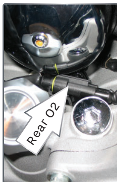
2007-2009 Touring and 2007-2011 Softail Models The stock O2 connectors for the front cylinder are found at the front of the engine near the voltage regulator. The stock O2 connectors for the rear cylinder are found at the rear of the engine near the oil tank.
