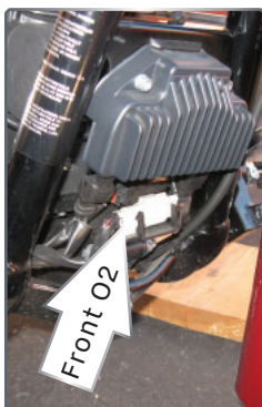
2006-2015 Dyna Models The stock O2 connectors for the front cylinder are found at the front of the engine near the voltage regulator. The stock O2 connectors for the rear cylinder are found under the seat.
