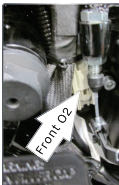
Street Models (500 and 750) The stock O2 connectors for the front cylinder are located on the right side of the bike between the swing-arm pivot shaft and the engine case. The stock O2 connectors for the rear cylinder are behind the left hand side cover above the coolant reservoir.
