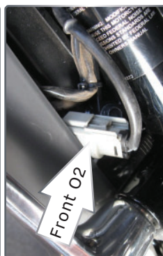
V-Rod Models The stock O2 connectors for the front cylinder are always on the left side of the radiator. You may need to loosen the radiator shroud to gain access to it. The stock O2 connectors for the rear cylinder are found under the seat near the fuel filler.
