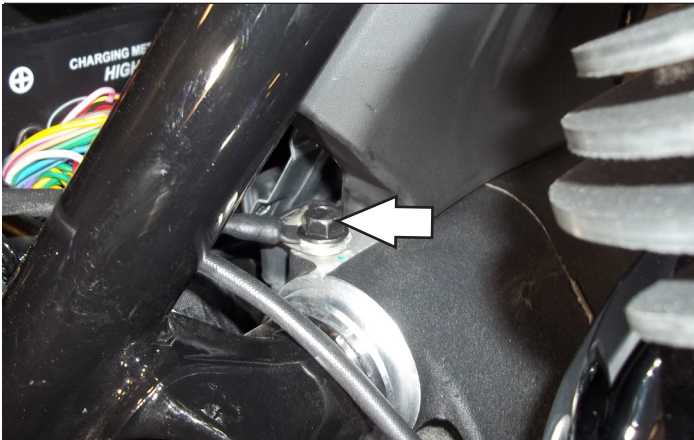
ATTACH GROUND WIRE
