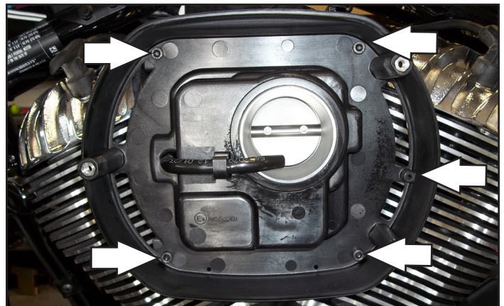
REMOVE BACKING PLATE
