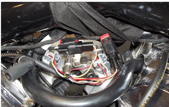
CONNECT TO INJECTORS
