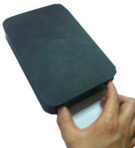
① Draw out the HDD bracket
