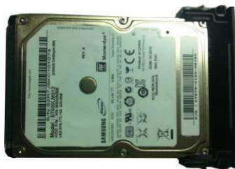
② Make sure the HDD metal surface is facing up and then put the HDD into the bracket
