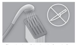
• Rinse the slots of the air cooler from the front side with running water.
