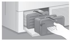
• Let the water drip off and put the air cooler back in place.
