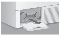
• Unlock the air cooler by turning the blue locking levers inwards.
